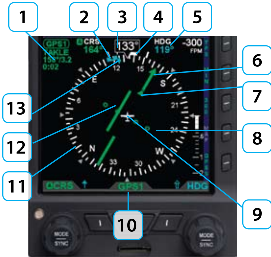
Figure 4-32 Horizontal Situation Indicator
