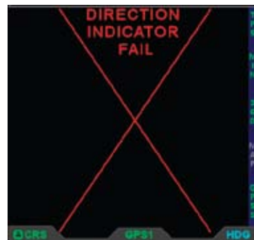
Figure 4-79 Direction Indicator Fail
